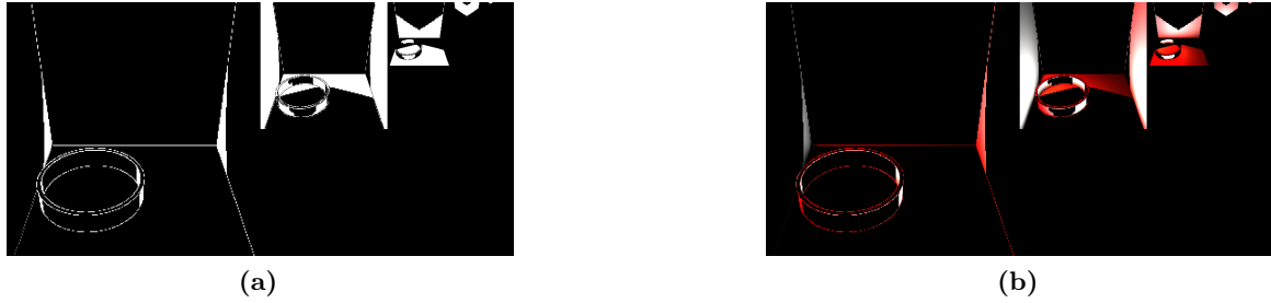
Figure 3.3: From left to right: Stencil marked multi-resolution regions and their shaded result. The white pixels on the left image correspond to the valid regions.
